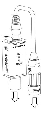
Insert *318BTS* into the audio mixer (Mic level), then connect the audio breakout cable supplied with the unit and insert the other end into a second channel on the audio mixer.
