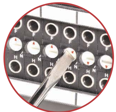
Easily Normal The Jacks By Rotating To "Full", "Non", Or "Half" Positions
