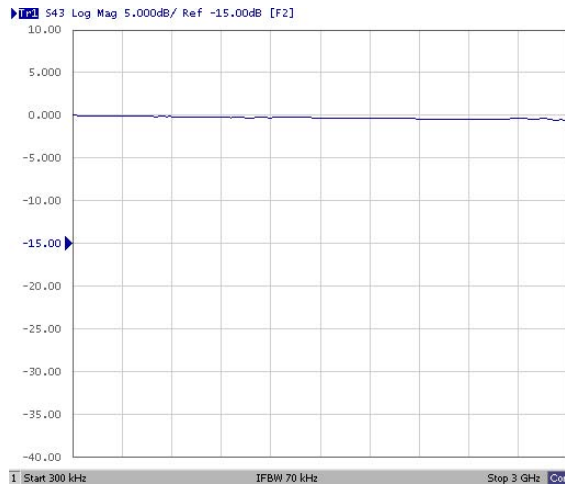
TYPICAL INSERTION LOSS FOR MVJ75TZ
