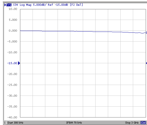
TYPICAL INSERTION LOSS FOR MVJS75T
