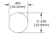
RECOMMENDED PANEL CUT-OUT TOLERANCE: ±.003
