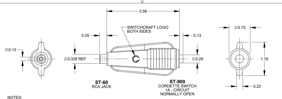
1. MATERIALS: CORDETTE SWITCH: HOUSING - THERMOPLASTIC, WHITE BUTTON - THERMOPLASTIC, BLACK CONTACTS - COPPER ALLOY, GOLD PLATED OVERMOLD - THERMOPLASTIC, GRAY
