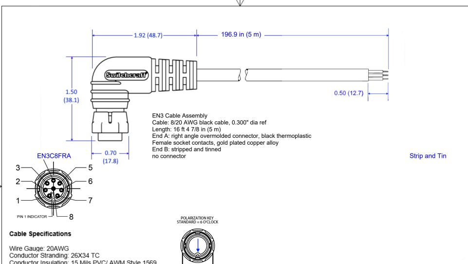
Conductor Insulation: 15 Mils PVC/ AWM Style 1569
