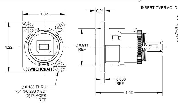
USB "A" CONNECTOR RETAINING NUT -USB "B" CONNECTOR STANDARD E SERIES HOUSING SEE TABLE FOR FINISH
