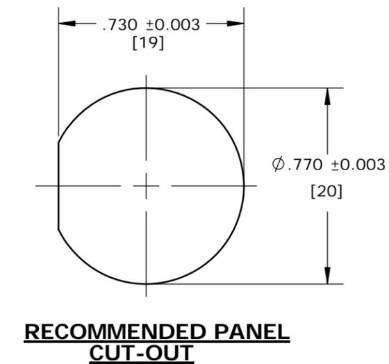
DIMENSION IN BRACKETS [] ARE METRIC, mm.
