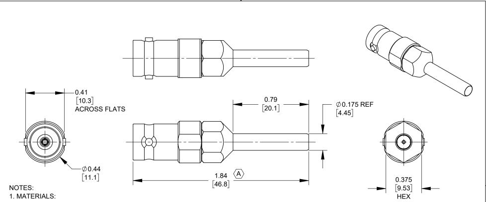
BARREL, SHELL - BRASS ALLOY, NICKEL PLATED MICRO CONTACT - BRASS ALLOY, GOLD PLATED BNC CONTACT - BERYLLIUM COPPER, GOLD PLATED INSULATORS - TEFLON
