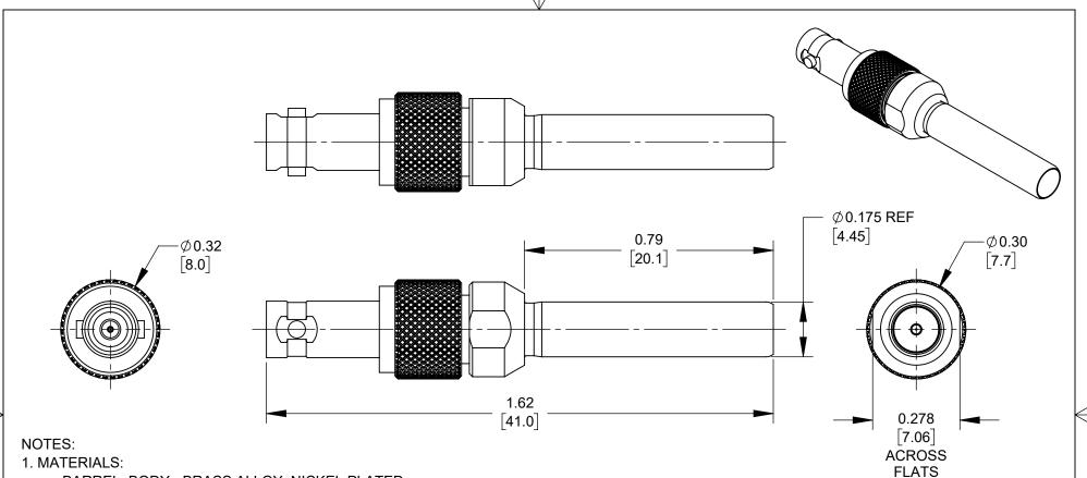
BARREL, BODY - BRASS ALLOY, NICKEL PLATED CONTACT - BERYLLIUM COPPER, GOLD PLATED INSULATORS - TEFLON
