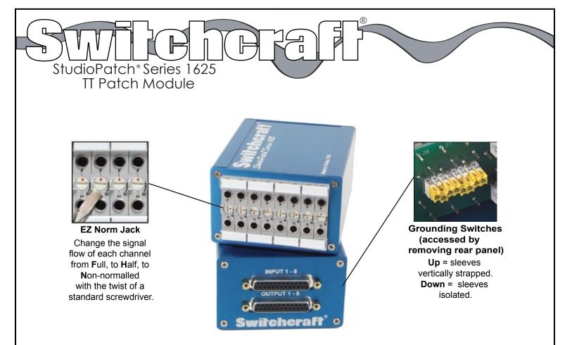
The 1625 utilizes EZ Norm technology, which allows signal flow to be changed from the front of each channel using a standard screwdriver. Additionally, programmable ground lift switches are easily accessed by removing the rear panel. Each module connects to your gear using two DB25 connectors wired to the TASCAM DTRS pinout.
