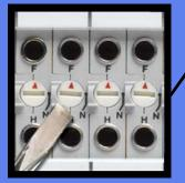
EZ Norm Jack Change the signal flow of each channel from Full, to Half, to Non-normalled with the twist of a standard screwdriver.
