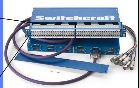
StudioPatch<sup>®</sup> Series audio patchbays utilize Switchcraft's EZ Norm technology, allowing signal flow to be changed from the front of the patchbay using a standard screwdriver. Now, every StudioPatch<sup>®</sup> Series patchbay comes with easy access programmable grounds, making it possible to custom configure the ground setting of each channel to either vertically strapped or isolated.
