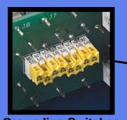
Grounding Switches Up = sleeves vertically strapped. Down = sleeves isolated.
