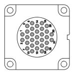
THREADED TYPE 5 KEY 31-POSITION #20 PIN CONTACT
